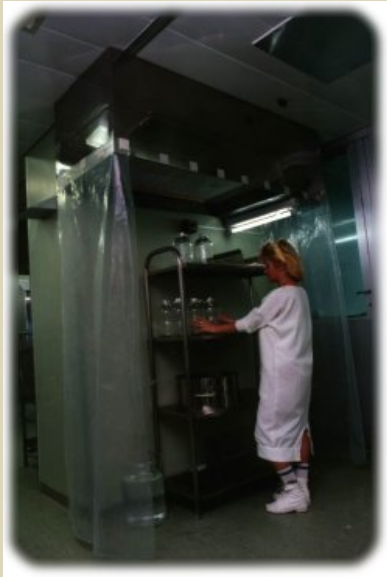
BV-1200 laminar flow cabinet The laminar airflow of the working area is classified into the 100 th class according to the Standard US209/E
