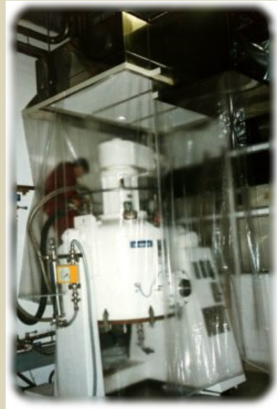
BV-1000x1800 laminar flow tent The laminar airflow of the working area is classified into the 100 th class according to the Standard US209/E
